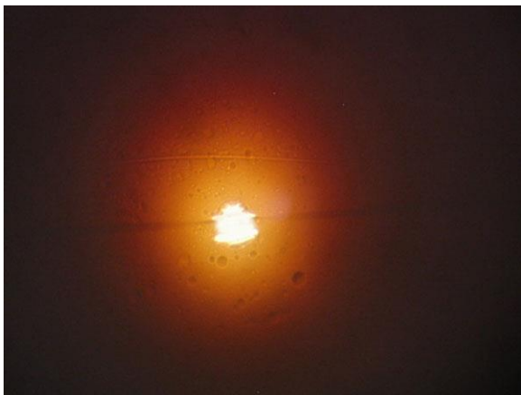
Fig. A: MAG*I*CAL ® Standard as shipped. Diameter of central perforation is ~ 0.1 mm
